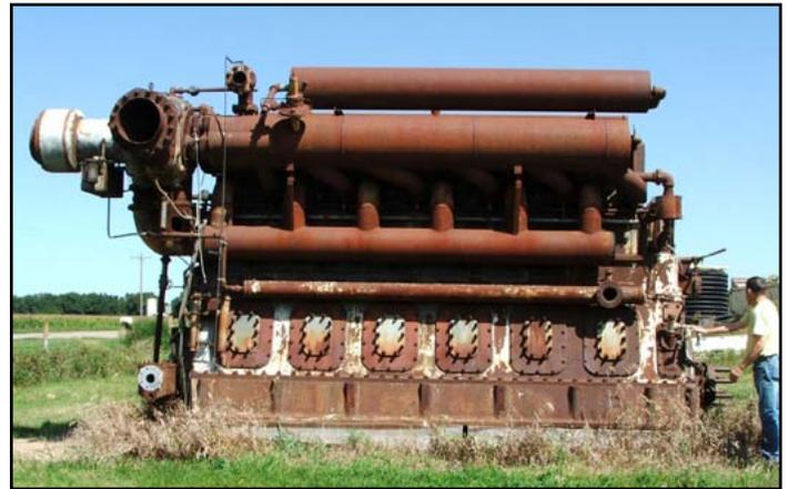
*The picture above is of the third diesel/natural gas engine purchased in 1945. This was a 1200 horsepower engine. This Worthington engine was 15'-7" long, 5'-3" wide and 11' tall. This mammoth was also six-cylinder. It produced 840 kilowatts at 1050 RPM. Note the relative size of the engine to the size of Gary standing off to the side.*
