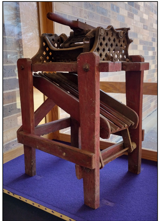
A 1900 era 39”-high potato cutter made by the Aspinwall MFC Co. in Jackson, Michigan. Although designed to cut potatoes for seed the potato cutter proved to be slow and cumbersome.
